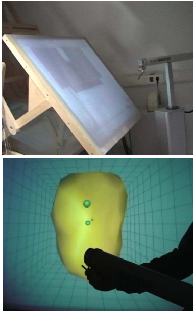
Figure 10: Hybrid Model. Two images of the simulator running in the workbench with the Fokker Haptic Master device.
